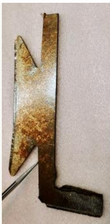
burned mica segment
