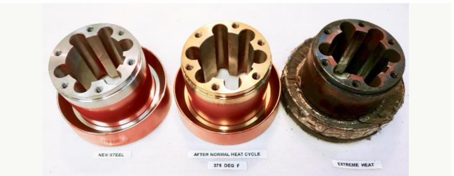
Pictured above: A steel part from a commutator that failed prematurely having clear signs of severe overheating resulting from a torch being used to expedite the installation process onto the armature shaft as evidenced by the uneven heating originating in bore on riser end in addition to a brand new steel part prior to normal oven cycles and a brand new steel part after completing multiple cycles of normal heating to 190°C/375°F. Please note, the overheated commutator in these images has not been in a burn-off oven. Using an oven for preheating might take longer, but it's vastly superior than risking premature commutator failure as a result of overheating.
