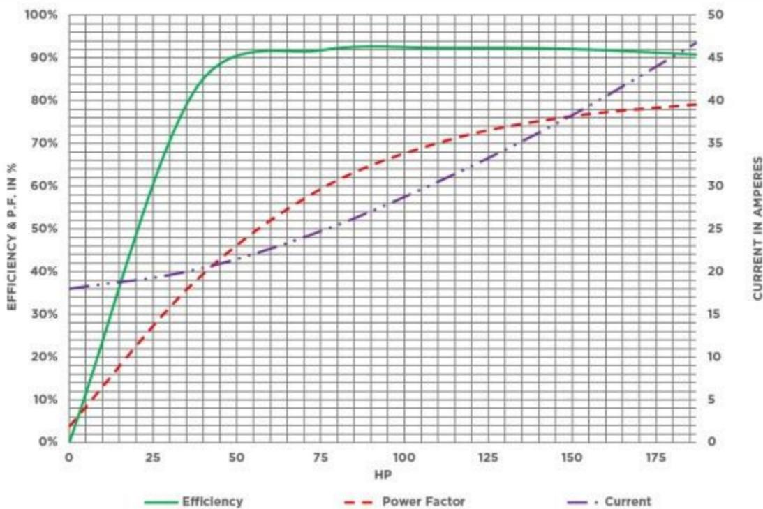
Figure 1 – Typical Eff/PF/Amps vs HP Curves for an Induction Motor (credit designmotors)
